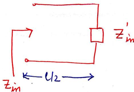
From the figure, it is clear that input impedance of a waveguide work as the load impedance of the another series connected waveguide.
